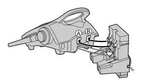
**4** Adjust the adaptor to hold the base unit, then push it in the direction of the arrow until it clicks into place.
