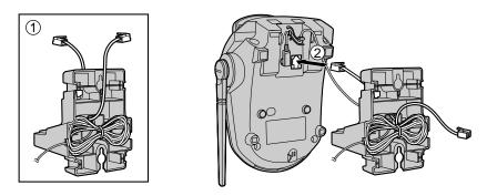
3 Insert (A) and (B) hooks on the wall mounting adaptor into the holes on the base unit.
